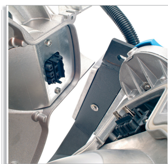
Built-in safety knife connector system, which automatically disconnects the mains power when the rear-access back cover is opened
